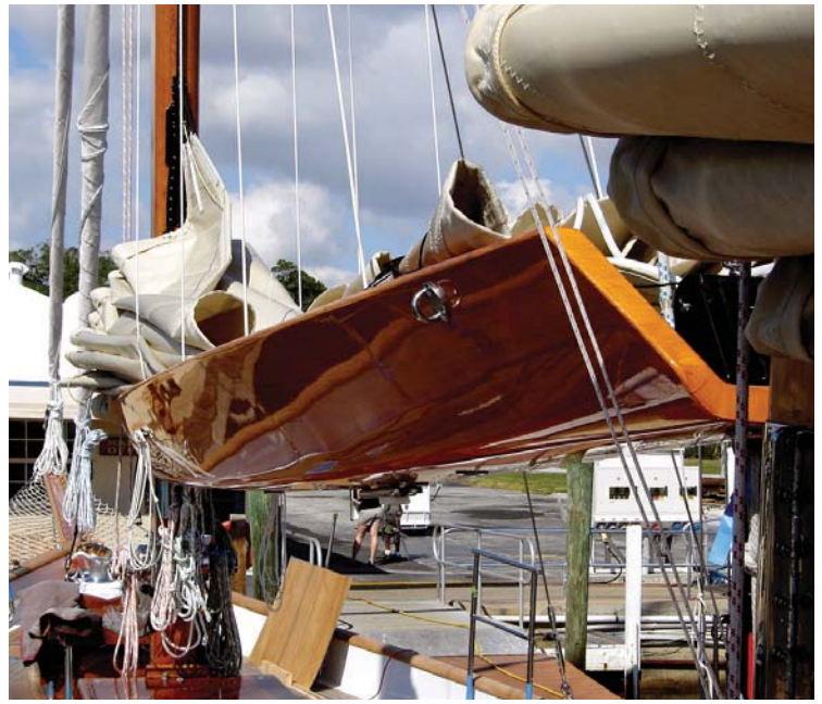
On SummerWind pocket booms allow long battens and make sail furling/stowing easy.
