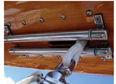
Top: Up close, can you tell what is wood? Bottom: Vang exits through slot in boom.
