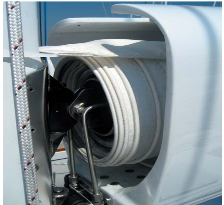
The hydraulic winding motor for furling the sail is inside the forward end of the mandrel.
