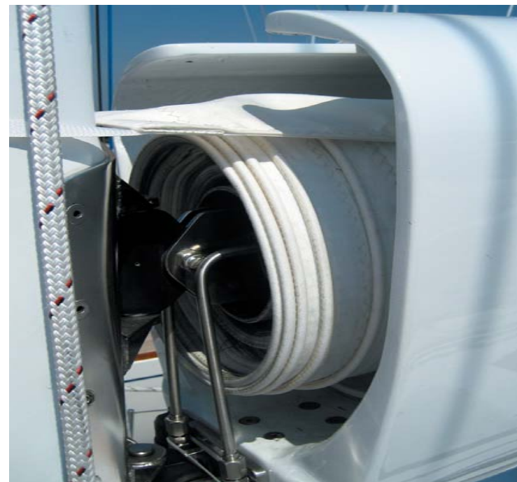
The hydraulic winding motor for furling the sail is inside the forward end of the mandrel.
