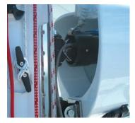
capability of our feeder design reduces binding and jamming, one of the biggest complaints that sailors have had with in-boom furling from other sources. With the motor located inside the mandrel, there's no need for an unsightly motor drum on the mast nor a strength-weakening shaft running through it.
