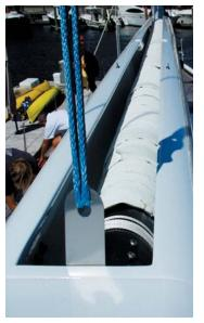
GMT's furling motor is easily accessible inside the boom's forward end. Many furling booms place their heavy motor at the aft end, requiring longer, heavier hydraulic lines and causing the boom to swing more violently in a seaway. Experienced sailors also favor in-boom furling to allow full-length battens for optimum sail shape and efficiency.
