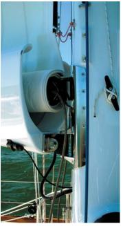
The forward end of GMT's PowerFurl boom is open. This feature allows no place for the sail to snag. The winding motor can be electric or hydraulic and is mounted inside the mandrel. You can completely furl your mainsail in less than 40 seconds with just the push of a button.
