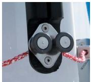
GMT uses a low-profile sail track which is less than a third the proud height of other furling boom systems' metal tracks. There's no setback or cutaway notch in the mainsail tack, and our articulating sail-feeder accepts mainsails with bolt-rope luffs, so that a racing sail can be used for both regattas and cruising. The angling
