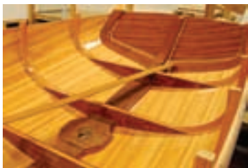
French & Webb's cold-molded hull.
