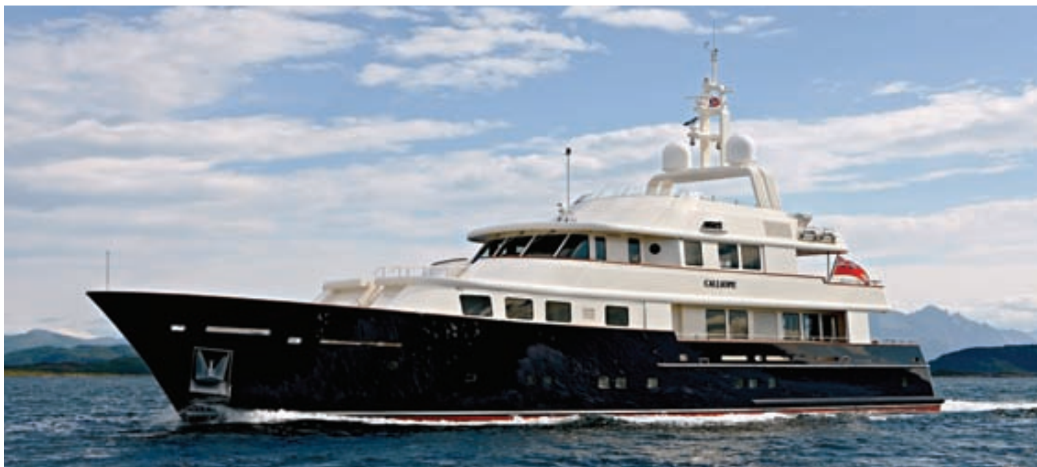
GMT's experience with carbon fiber led to Langan Design selecting us to fabricate the custom arch which supports navigation and safety gear on the award-winning superyacht Calliope.
