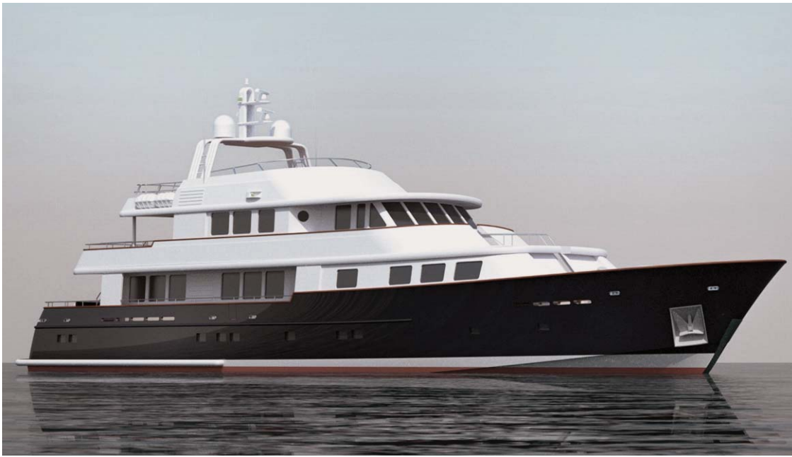
A classically-styled superyacht whose topline is enhanced by a structural arch which supports her electronics gear.
