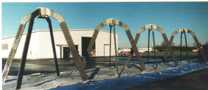
QUADRUPEDS USED TO SUPPORT INSTRUMENTS AT THE FOCUS OF THE ANTENNA BUILT FOR THE HARVARD SMITHSONIAN ASTROPHYSICAL OBSERVATORY. THE QUADRUPED AND HUB ARE PART OF THE RADIO TELESCOPE ARRAY OF WHICH SEVERAL WERE BUILT AND DEPLOYED FOR DEEP SPACE EXPLORATION. GMT WAS CITED BY THE SAO AS THE BEST OUTSIDE CONTRACTOR WORKING ON THIS PROJECT.
