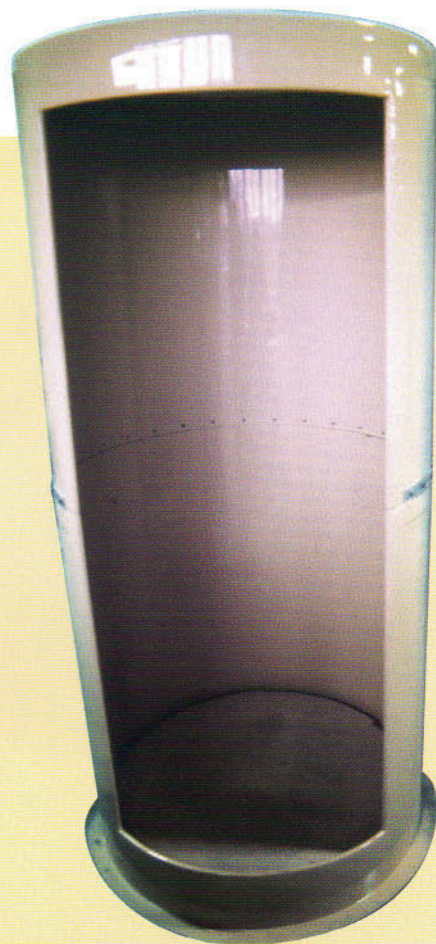
"ROBO TUNA" IS A SUBMERSIBLE BUILT FOR DRAPER LABORATORIES AS PART OF THEIR INVESTIGATION FOR ALTERNATIVE PROPULSION. GMT PROVIDED THE BODY, WHICH WAS VERY ACCURATELY MODELED AFTER A TUNA FISH. DRAPER FITTED A SOPHISTICATED TAIL WITH THE HOPE OF PRODUCING A HIGHLY ENERGY EFFICIENT MEANS OF PROPELLING UNDER WATER VEHICLES.
