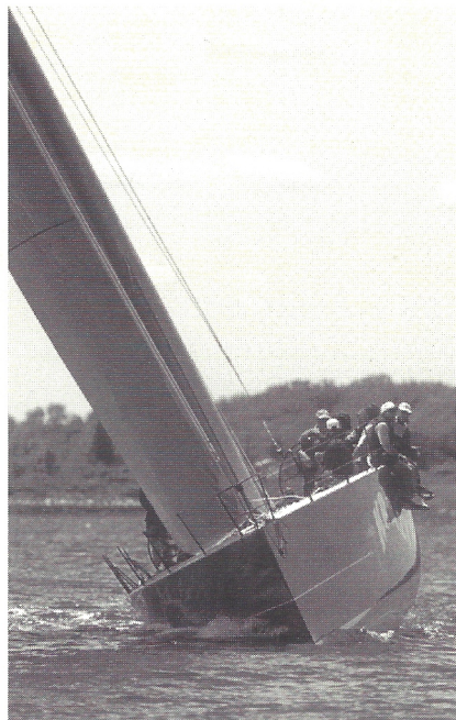
Beating to weather Crazy K-Yote Two's GMT built free standing carbon wing mast provides optimal headsail sheeting angles and fast tacks.
