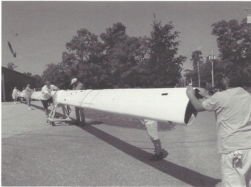
GMT's longest spar yet, 124 ft. B&R rigged mast for the Rivolta 90 leaves the paint shop. The spar is scheduled to join the boat in December, 2000.
