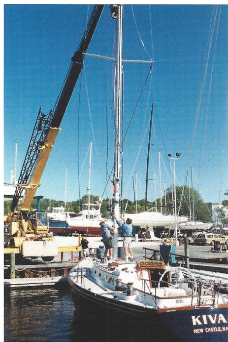
New GMT spar being installed in KIVA, Hinckley Sou'wester 51-01 in time for the "Thrash to the Onion Patch."
