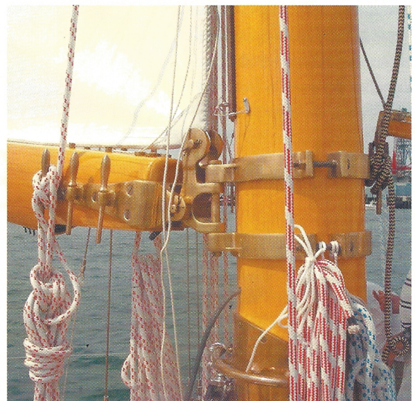
LION'S WHELP's main boom outboard end features a custom bronze cap with sheet and preventer attachment points as well as a stylized lion's head. Main mast detail showing bronze gooseneck hoops and inboard boom end belaying pins.
