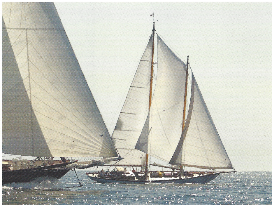
LION'S WHELP , 65 ft. Alden schooner built by Portland Yacht Services, features all carbon spars by GMT Composites and is shown racing in the 2003 Shipyard Cup alongside the 107 ft. wishbone ketch SINTRA .
