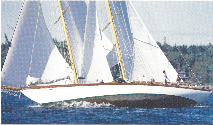
GMT's carbon fiber "Faux Bois" spars lend strength and beauty to LION'S WHELP's cloud of canvas as she sails to weather during the Shipyard Cup.
