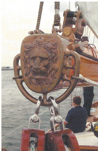
LION'S WHELP's main boom outboard end features a custom bronze cap with sheet and preventer attachment points as well as a stylized lion's head. Main mast detail showing bronze gooseneck hoops and inboard boom end belaying pins.
