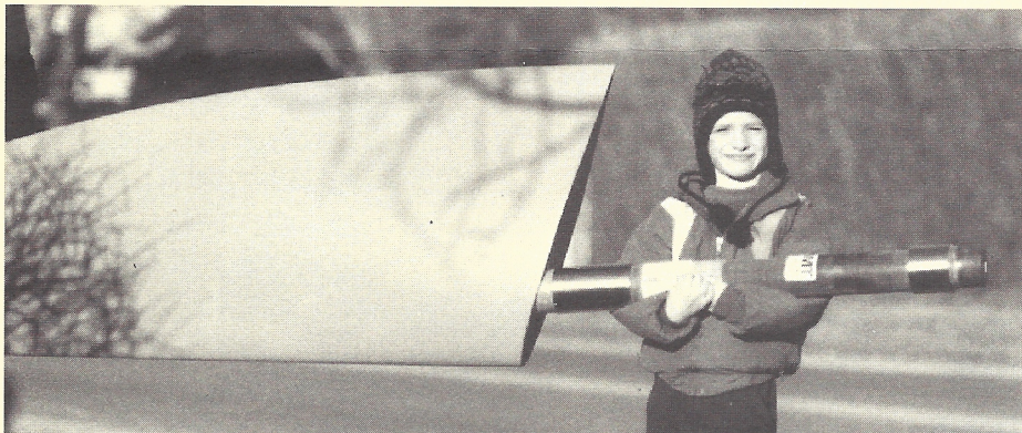
8 year old Nicholas Walton demonstrates the versatility of carbon fiber with this 22 lb rudder for their Hinckley 41
